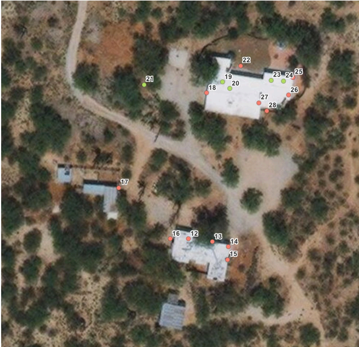
Figure 4. Fixture Compliance with Dark Sky Guidelines for Visitor Center Area Bollards. Dark sky compliant lighting has a green marker and non-compliant lighting has a red marker.
