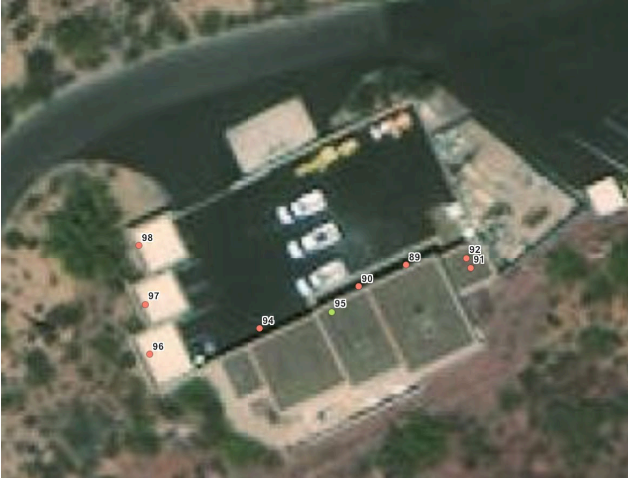
Figure 12. Fixtures Identified within the Tucson Mountain District Maintenance Area. Dark sky compliant lighting has a green marker and non-compliant lighting has a red marker.
