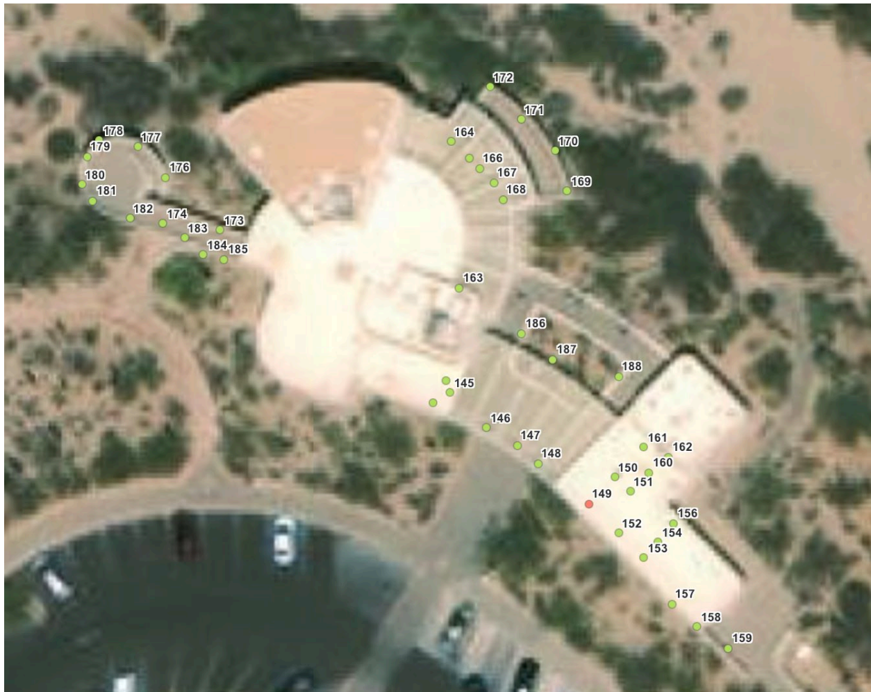
Figure 15a. Fixture Compliance with Dark Sky Guidelines for the Red Hills Visitor Center Building. Dark sky compliant lighting has a green marker and non-compliant lighting has a red marker.
