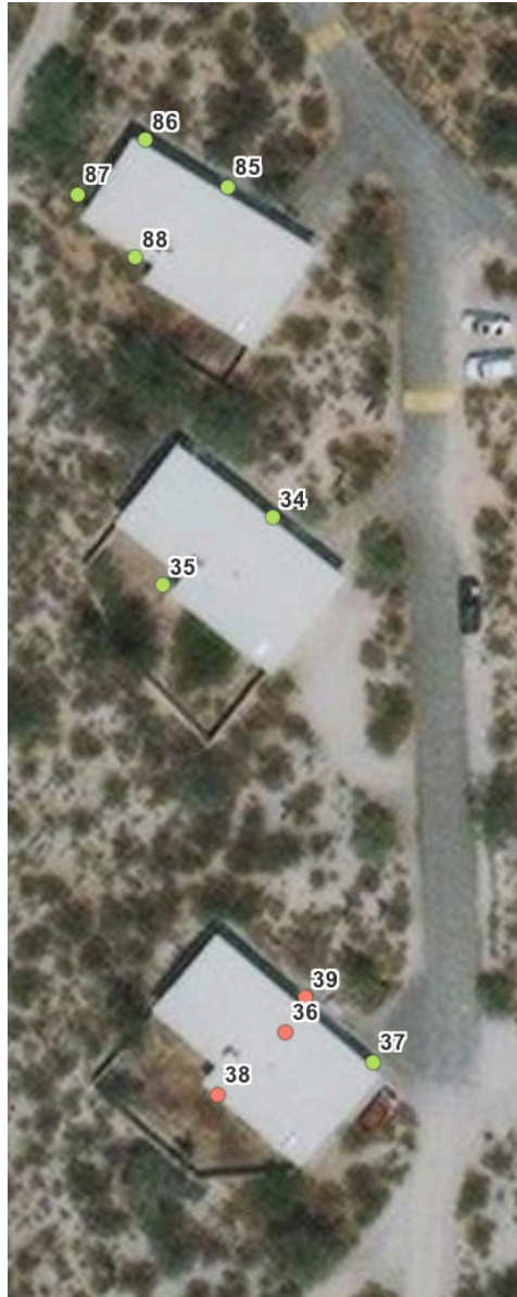
Figure 6. Fixture Compliance with Dark Sky Guidelines for Quarters 14, 15, and 16. Dark sky compliant lighting has a green marker and non-compliant lighting has a red marker.
